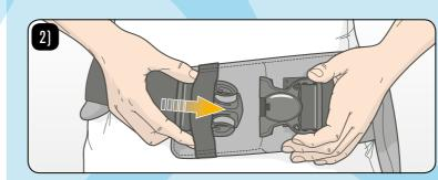
Then guide the male part of the buckle through the elastic safety loop and fasten the buckle. The buckle has been properly fastened when you hear a loud "clicking" sound and the clasps on both sides have snapped into place.
