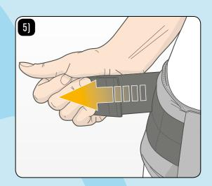
Now adjust the short end of the webbing such that the buckle is positioned behind the safety loop and on top of the padding.
