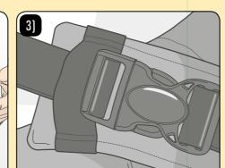
Ensure that the buckle is positioned behind the elastic safety loop.
